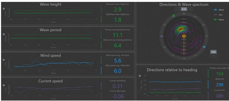
Through robust, accurate and adaptive algorithms the Wavex calculates directional wave, surface current, and speed through water data. It will interface with a variety of X-band radars, including a ser of IP radars, without interfering with, or affecting the navigation system. Wavex requires at least 1-3 m/s wind. Heavy precipitation will affect data capture rate.
