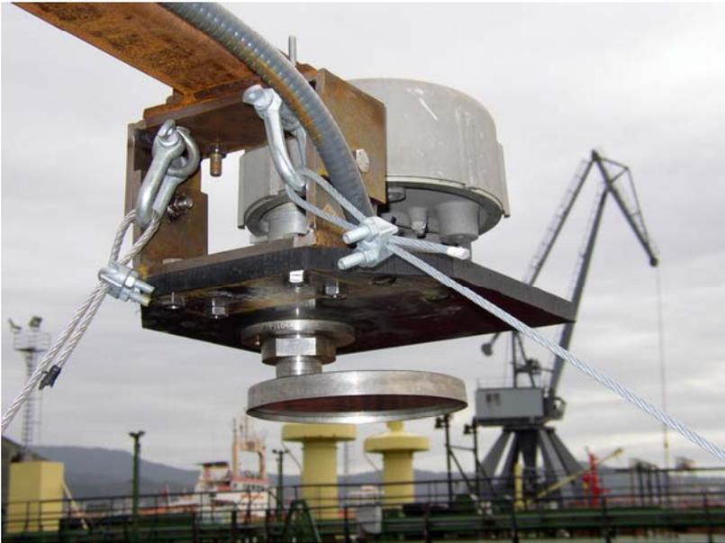
Figure 5 Horn antenna of the RADAC tide gauge.
