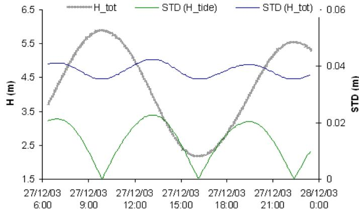
**Figure 23** Theoretical evolution of the STD for a tidal curve with (green line) and without waves (blue line). The evolution of the sea level is also presented as a reference (in grey, thicker line).
