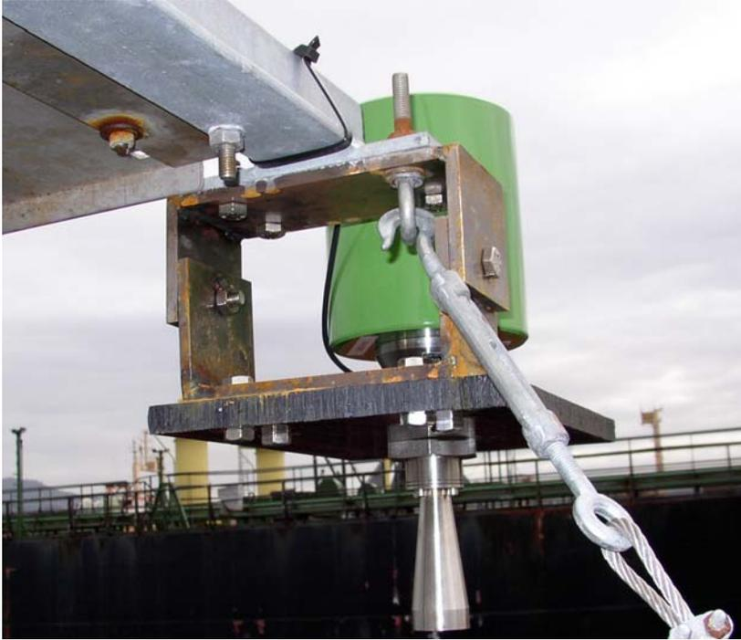
Figure 7 Horn antenna of the SEBA tide gauge.
