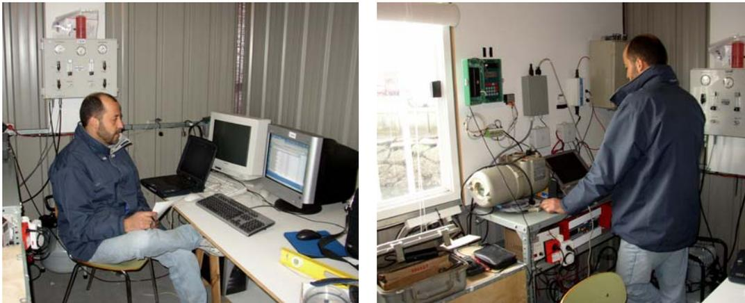
**Figure 11** Interior of the hut with the computers and the rest of the electronic devices for the tide gauges.
