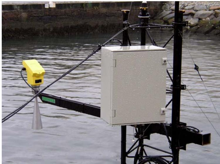
Figure 2 Horn-antenna and box containing the datalogger for the GEONICA system
