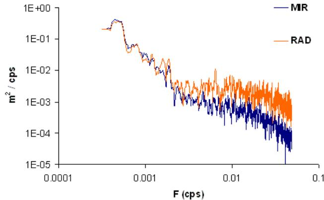
Figure 19 Comparison between the power spectral density of the raw 1s time series provided by MIR and RAD
