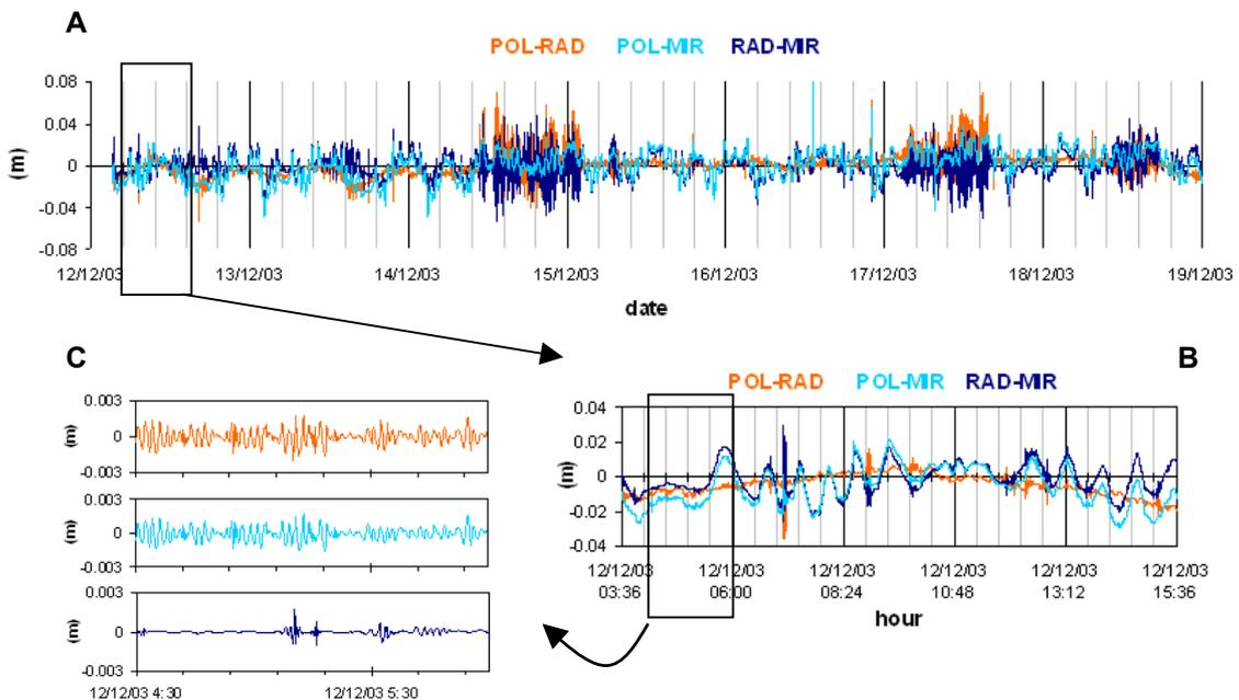
**Figure 20 Evolution of the differences between the data provided by POL, RAD and MIR (averaged each 10 s) during one week (A) and during one day (B) and one hour (C). See text for details.**
