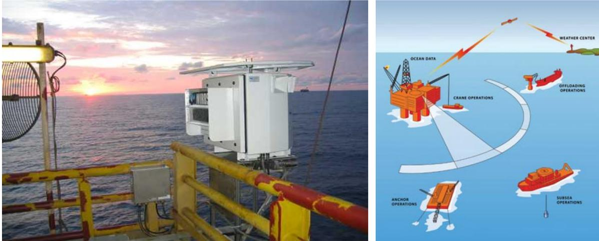
Fig.2: Microwave Doppler radar providing wave and surface current data
