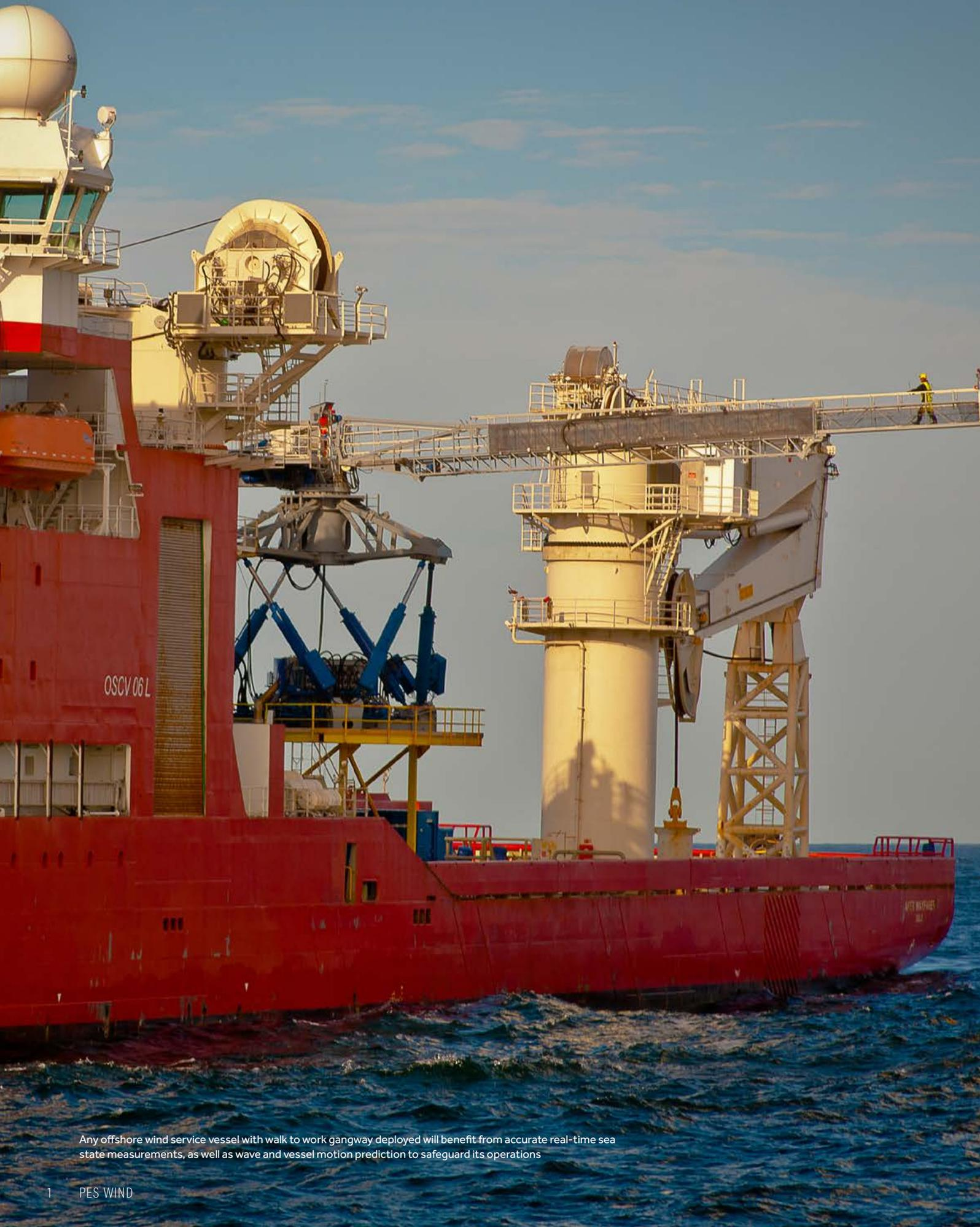
Any offshore wind service vessel with walk to work gangway deployed will benefit from accurate real-time sea state measurements, as well as wave and vessel motion prediction to safeguard its operations
