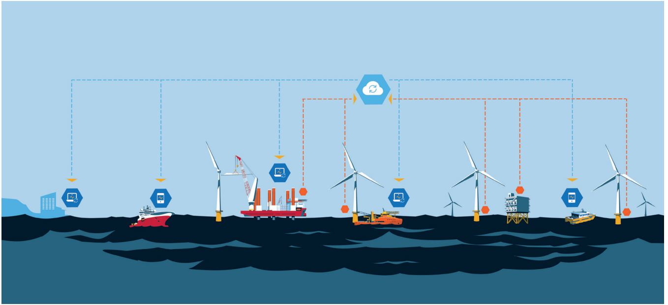
Miros sensors are radar-based, dry IoT sensors providing reliable, highly accurate, real-time measurements of the ocean state to enhance safety, efficiency, and performance of operations while reducing costs during the lifecycle of an offshore wind farm.
