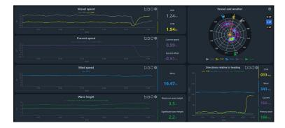
The Miros WaveSystem combines measurements from two different sensors - the X-band radar-based Miros Wavex and the downward-looking Miros RangeFinder.
