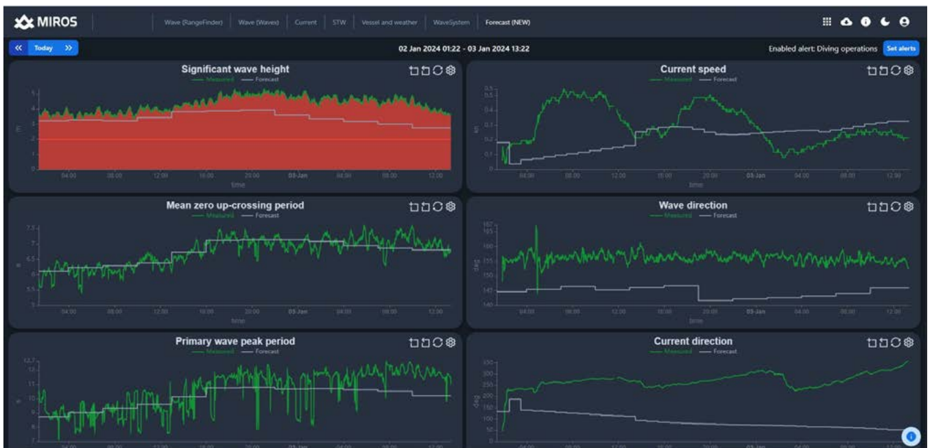
Enhancing maritime safety and operational efficiency, the Miros Forecast app integrates ocean condition forecasts with real-time measured ocean data, visualizing the comparison in an intuitive and dynamic dashboard for better decision-making
