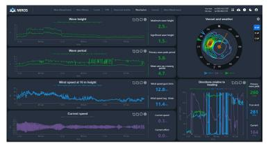
The Miros WaveSystem combines measurements from two different sensors - the X-band radar-based Miros Wavex and the downward-looking, DNV alpha-factor approved Miros RangeFinder.
