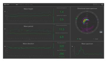
The Miros Wave & Current Radar observes the ocean surface in a semi-circle at a distance of 180 - 450 m depending on the installation height, typically 18 - 80 m. The radar frequency gives a strong echo from capillary waves which are normally present at wind speeds > 2 m/s.
