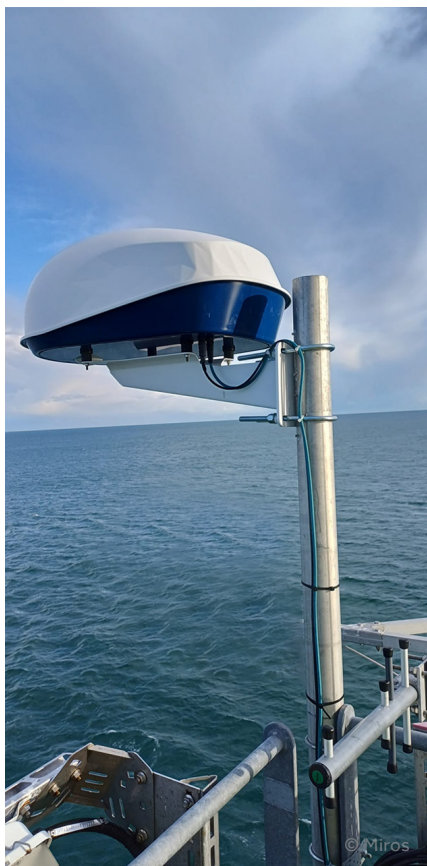
Miros WaveFusion sensor installed on a turbine. Miros' real-time metocean measurement systems have been rigorously tested across the world's harshest offshore conditions and are ready to be retrofitted to existing infrastructure
